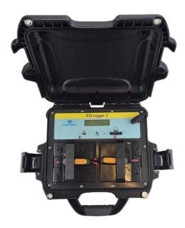
The IFQ LOGGER 2 is a portable converter and data logger designed for use with Flow-Tronic flow sensors. It is equipped with one RS485 digital serial communication port for RAVEN-EYE®, RAVEN-EYE® 2(+), BELUGA, BELUGA A/V or PHOENIX 2 sensors, along with a 4–20 mA input for external level measurement.
